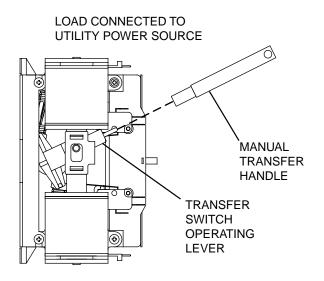
utility source voltage is available to the standby closing coil terminals, but transfer to Standby does not occur, the cause of the failure may be (a) a failed standby closing coil and/or bridge rectifier, or (b) a seized or sticking actuating coil or load contact. This test will help you evaluate whether any sticking or binding is present in the transfer mechanism.
